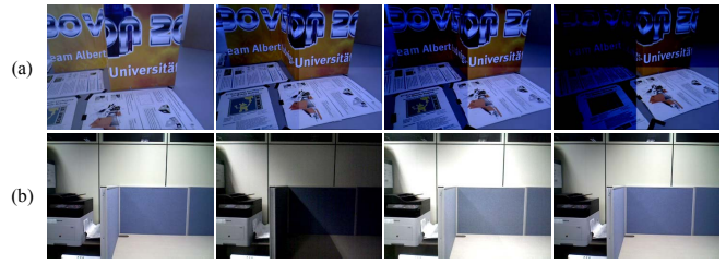
Fig. 6. The RGB image sequences in synthetic & author-collected RGB-D dataset. (a) To simulate irregular illumination changes, we manipulate the intensity values of the images in TUM RGB-D dataset based on four different illumination change models. (b) The images are captured in a stationary position with calibrated Asus Xtion Pro Live RGB-D sensor. To test the robustness to illumination changes of each method in real world, lights in the room are turned on and off repeatedly by author.
