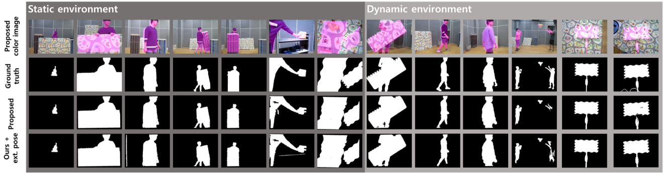
Fig. 5: Segmentation result for tested sequences in the order shown in Table.I. The first row shows the masked image and the second row represents the ground truth. The result of the proposed method with VO and external pose estimation is presented orderly in the third and fourth rows (except the TUM dataset for the reasons described in text). Since the depth is not measured on the boundary of the image, moving objects are not labeled in those areas.
