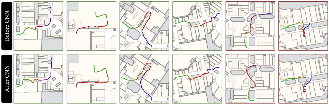
Fig. 5. Floorplan fusion by CNN. The top and the bottom shows the trajectories (time coded by color, blue→red→green) before and after the CNN application, respectively. CNN is effective in avoiding collisions with walls or inaccessible areas (first 4 columns). The last two columns show failure cases due to large initial alignment errors.
