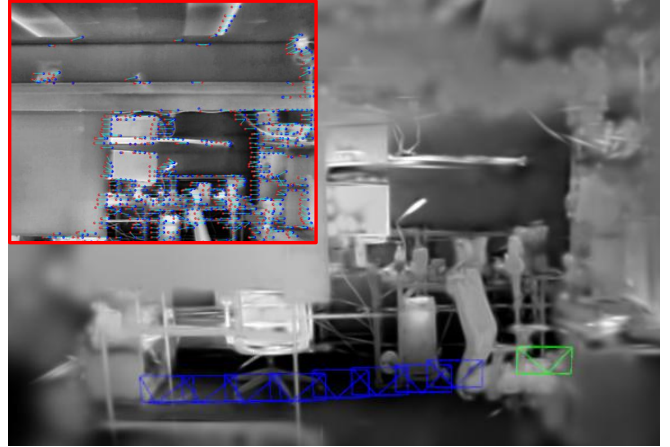
Fig. 1. Overview of PI-EAT-SLAM on the custom dataset, demonstrating robust tracking and mapping in low-contrast, texture-sparse thermal imagery. (Background) Overall visualization of the 3DGS mapping and camera trajectory. (Red box) Robust edge point matching for tracking: red and blue dots denote edge points extracted from the rendered and ground-truth images, respectively, with cyan lines indicating the residual vectors.
